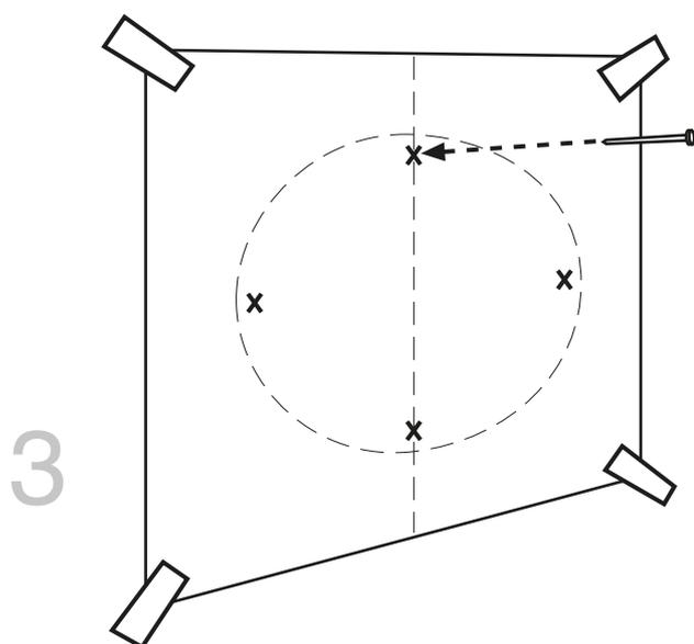
Then align the drilling template in the wished position,
