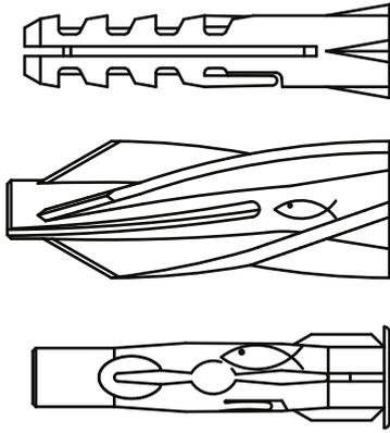
The enclosed pegs are standard pegs and are suitable for the attachment in massive walls made out of stone.
