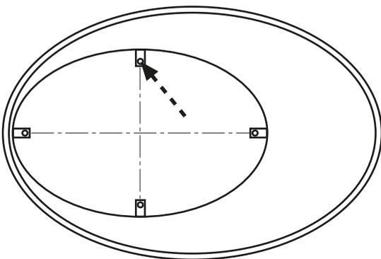
For reasons of production, with the models RONDO WALL Leather and RONDO WALL Felt the cover are produced with a little bit at the end which is closest to the wall. To compensate this the distance sleeves should be placed between the mounting lashes and the wall.
